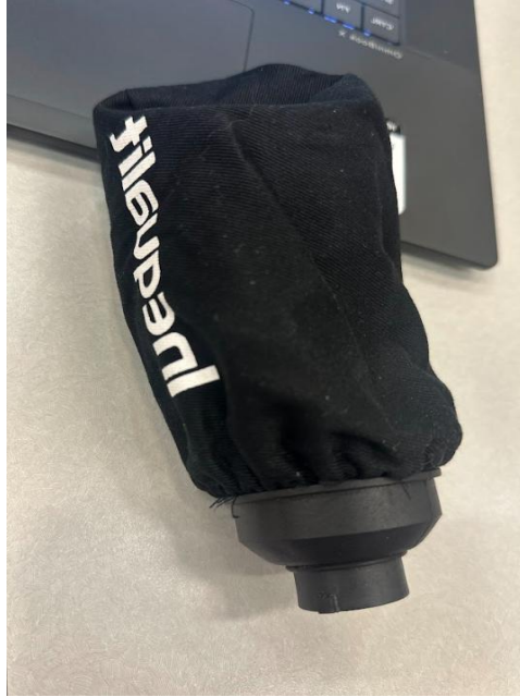
Figure 13. Dust Extraction Unit
